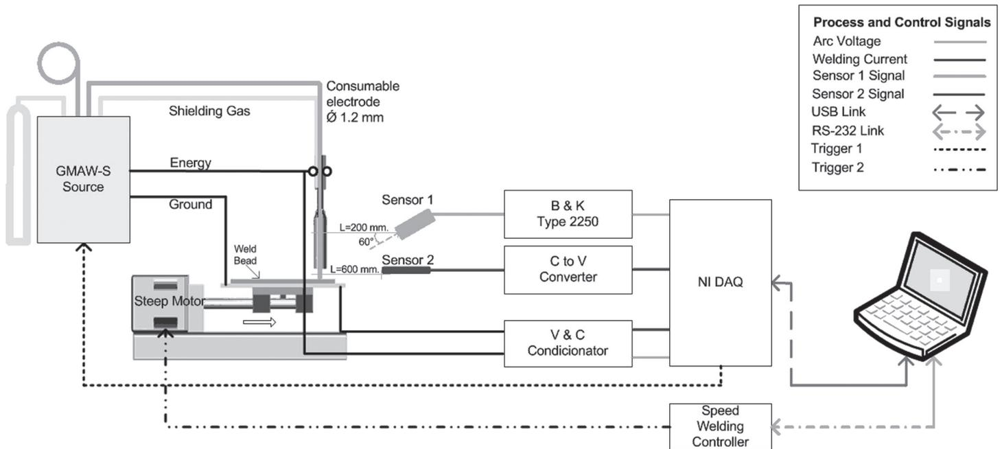
Figure 6. Experimental setup.
