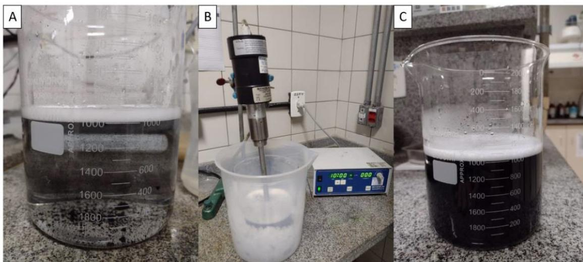
**Figure 3.** Dispersion process of carbon nanotubes. (A) Addition of the nanotubes to the solution before the ultrasound; (B) Solution in a temperature-controlled container for use in ultrasound; (C) Solution after 10 minutes in the ultrasonic homogenizer.
