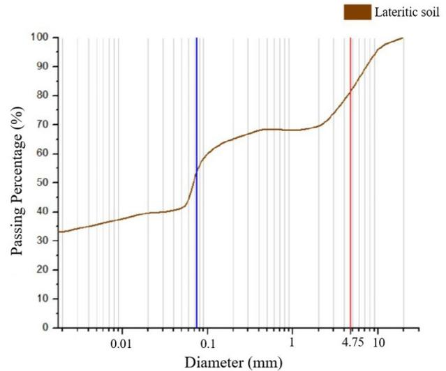
Figure 5. Graph of soil granulometry.
