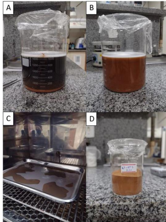
**Figure 4.** Process of preparation of samples used for physical and mechanical tests. (A) Addition of soil to the solution, before the agitator; (B) Soil solution + nanotubes after the shaker; (C) drying the solution in an oven; (D) Sample to be used in physical.
