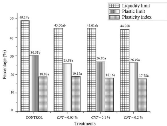
**Figure 13.** Averages of the Atterberg limits for the samples (control groups and with different additions of CNTs). Obs: Groups with the same letter do not differ significantly in relation to their means, according to the Tukey Test ( $\alpha = 5\%$ ).
