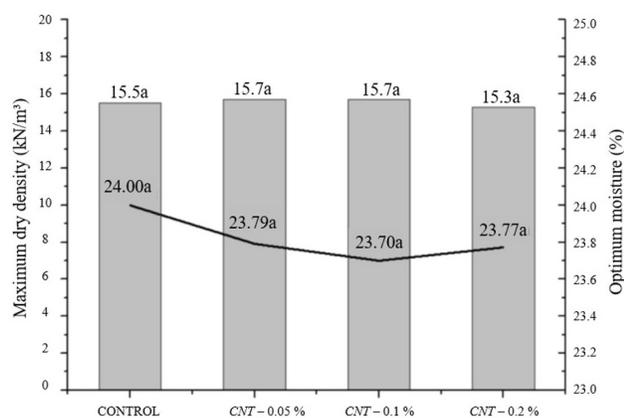
**Figure 16.** Means of maximum dry densities and optimal moisture of soil samples (control groups and with different additions of CNTs). Obs: Groups with the same letter do not differ significantly in relation to their means, according to the Tukey Test ( $\alpha = 5\%$ ).
