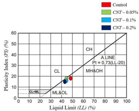
**Figure 14.** Sample results with CNTs according to USCS.
