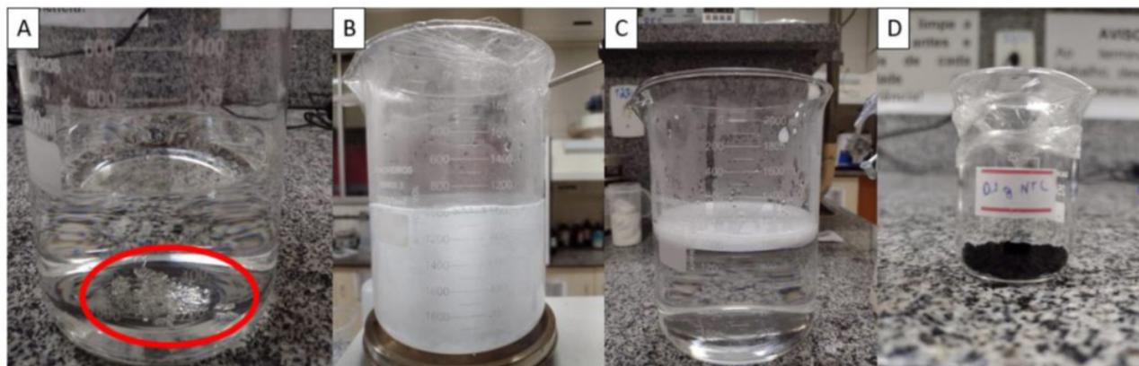
**Figure 2.** Solution for carbon nanotubes dispersion. (A) Solution with Tween 80 surfactant (before the shaker); (B) Solution during magnetic stirrer; (C) Solution after 2 h period on shaker; (D) Nanotubes used in the solution.
