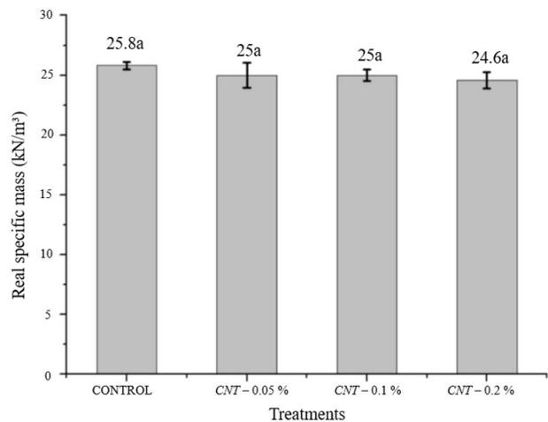
**Figure 15.** Averages of the real specific mass of the samples of the control groups and with different additions of CNTs. Obs: Groups with the same letter do not differ significantly in relation to their means, according to the Tukey Test ( $\alpha = 5\%$ ).
