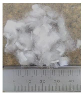
Figure 2. Polypropylene fibres.
