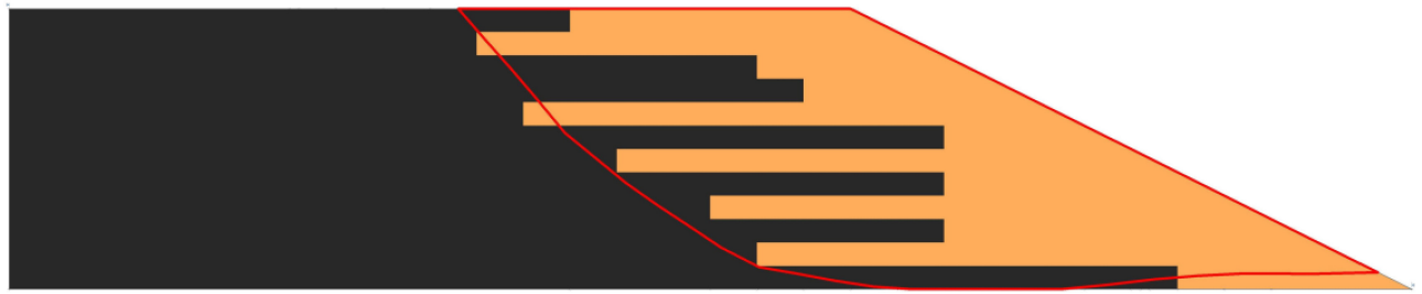
Figure 2. Example of a 2D component cross-sections analyzed ( F_{2D} = 0.994 ), black region is the inner material ( c_u = 60 kPa), the orange region is the outer material ( \phi' = 31^\circ , c' = 10 kPa) and the red line is the critical slip surface found.
