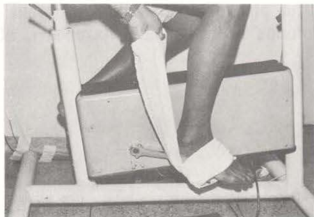
Figure 1 — Device used in order to avoid the retrograde movement of the pedal of the ergometric bicycle.
