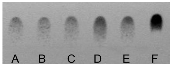
Fig. 1 – TLC plate developed in ninhydrin for glycine analysis. A, B, and C are glycine samples synthesized from 50, 100, and 150 ml ammonia, respectively. Sample D refers to ^{15}\text{N} -enriched glycine. E and F correspond to the glycine p.a. standard.
