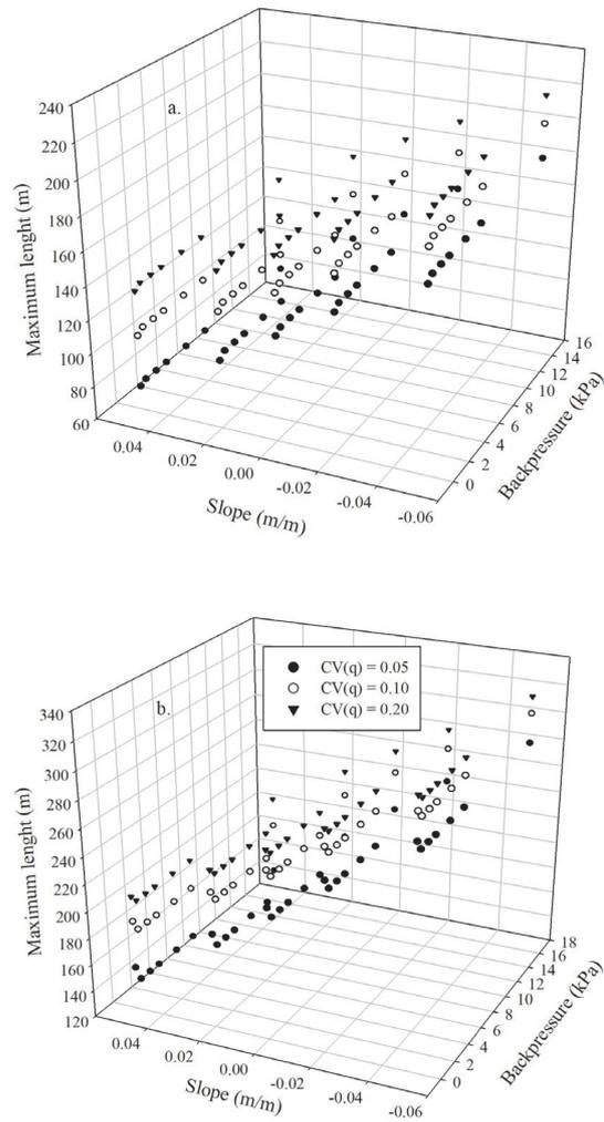
**Figure 1. Maximum lengths of the TalDrip (a) and D5000 (b) lateral driplines in surface and subsurface applications with an operating pressure of 145 kPa for different flowrate coefficients of variation, slopes and backpressures.**
