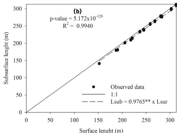
**Figure 2.** Correlation between the maximum surface and subsurface lengths obtained for the TalDrip (a) and D5000 (b) driplines under the different evaluated scenarios.
