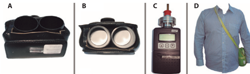
Figure 4. A) Double passive NO 2 sampler containing a cellulose filter (Energetica, Rio de Janeiro, Brazil) impregnated with an absorbent solution of 2% triethanolamine, 0.05% o -methoxyphenol, and 0.025% sodium metabisulfite inside a small plastic tube with one of its extremities open to ambient air. The nitrite produced during sampling is determined colorimetrically by reacting the with sulfanilamide and 8-anilino-1-naphthalene-sulfonic acid (ANSA) and monitoring the absorption at 550 nm wavelength; B) Superior view of the NO 2 sampler; C) Portable gravimetric impactor with a flow rate of 1.8 L/min. Air is aspirated into the impactor by a pump, PM is retained by a filter, and the particles in suspension in the air are measured gravimetrically; D) Portable sampler carried in a small bag by a research subject.
