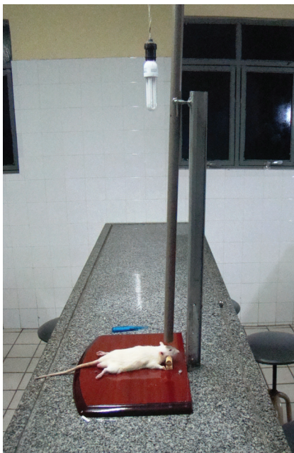
FIGURE 1 - Controlled falling weight closed head injury platform. A. Metal rod to support the driving weight duct. B. Driving weight stiff plastic duct (perfect metal sphere of known weight) measuring 1m of height. C. Platform basis for positioning the experimental animal with a head solid support.
