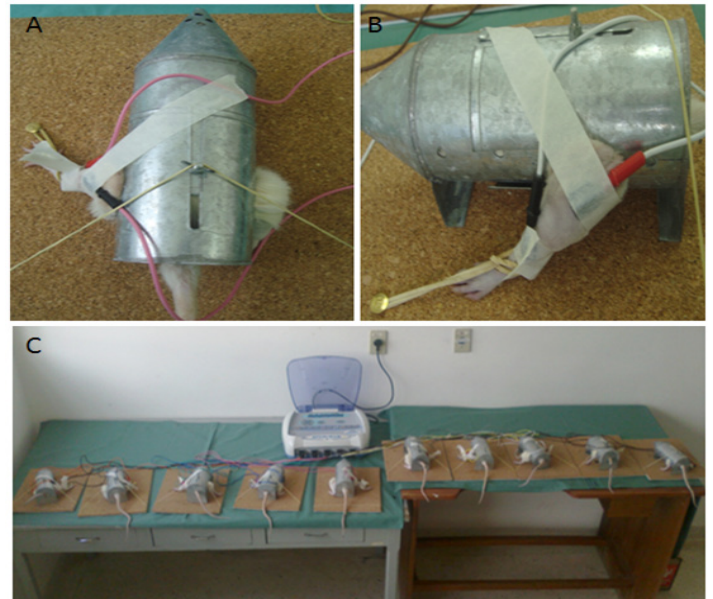
FIGURE 3 - Electrical Stimulation. A) Positioning of rats in capsule stimulation. B) Another view of the rats in the capsule. C) Rats receiving stimulation at the same time.
