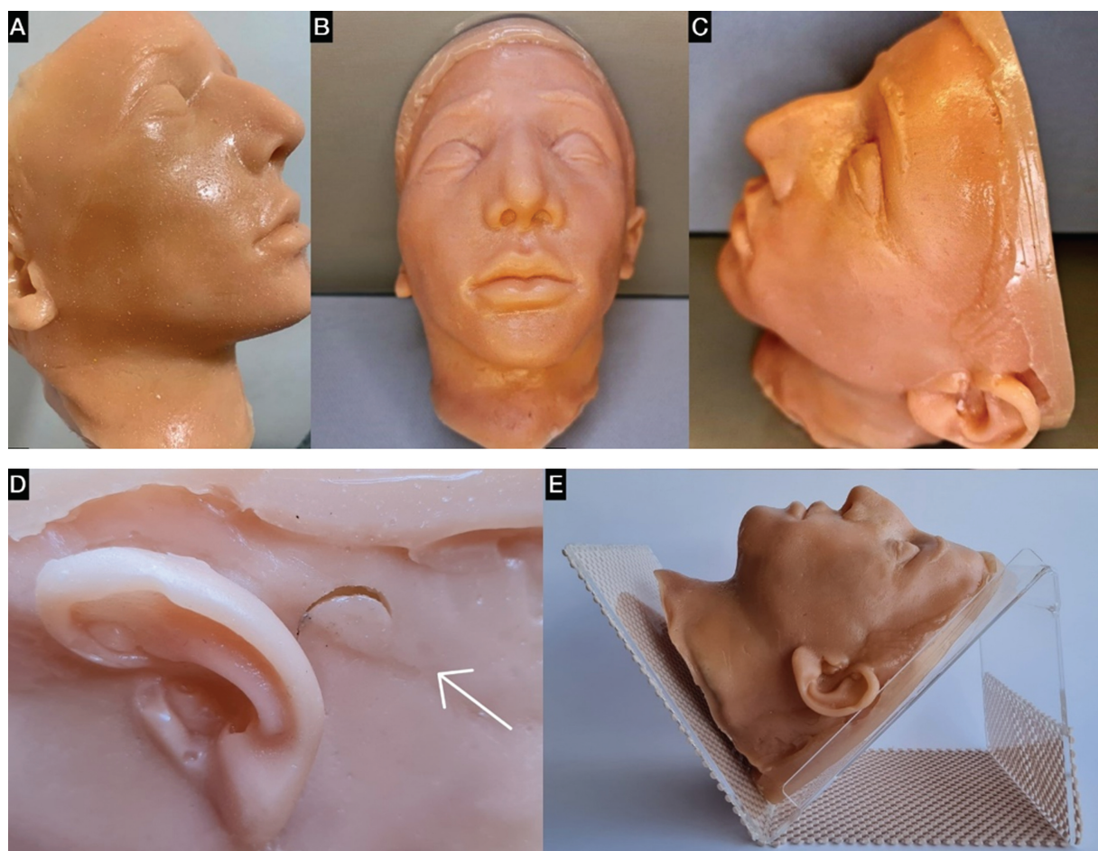
Figure 1 Anthropomorphic facial and cervical simulator. (A, B, C) Customized mannequin with external anatomical markers for facial characterization. (D) Monoblock model with elastomer skin, gel elastomer subcutaneous tissue, and polyurethane bone structure layers. Retroauricular drainage points. (E) Acrylic base with non-slip rubber fabric for stable positioning in supine or sitting positions.
