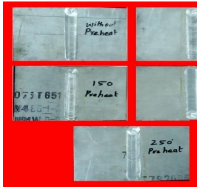
Fig. 2 Photograph of fabricated joints.
