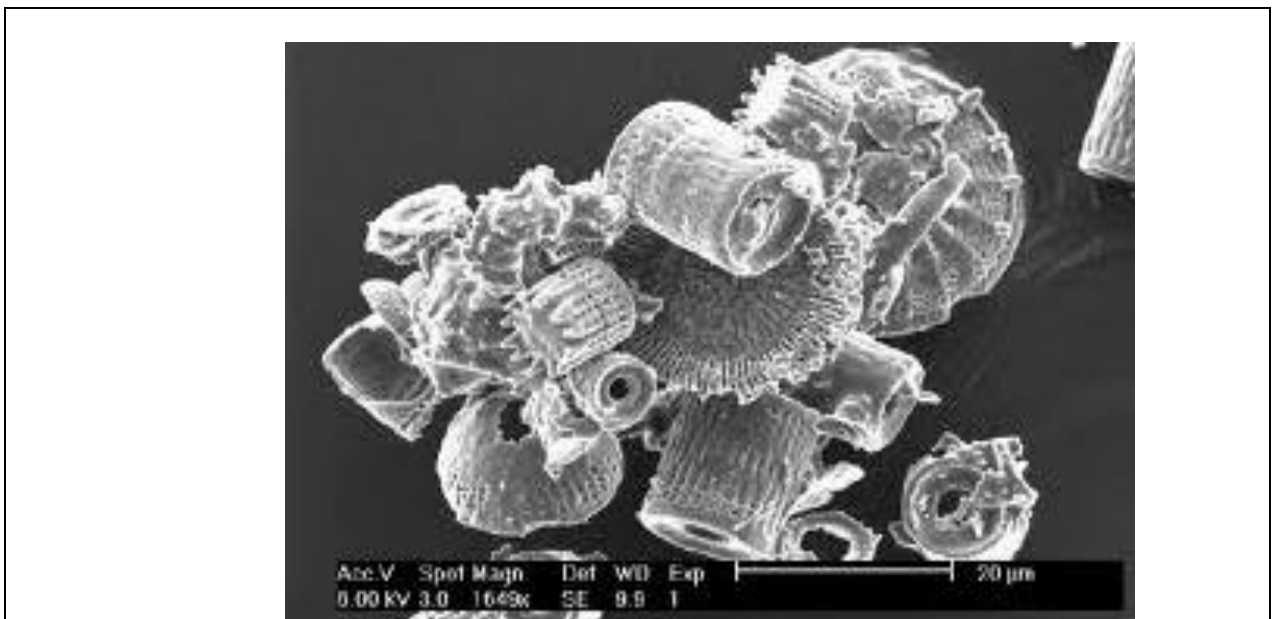
Fig.3 Diatomaceous earth as viewed under bright field illumination on a light microscope.
