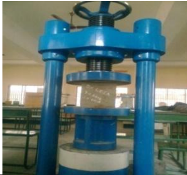
Fig.5 Compression Test on Cube
