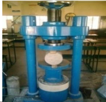
Fig.6 Split Tensile Test on Cylinder
