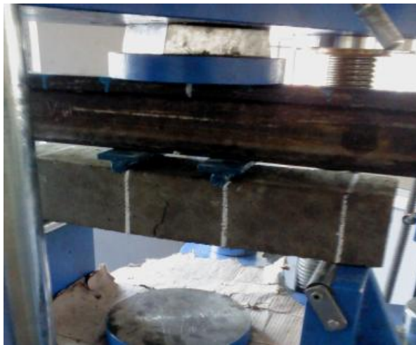
Fig.7 Flexural Test on Prism
