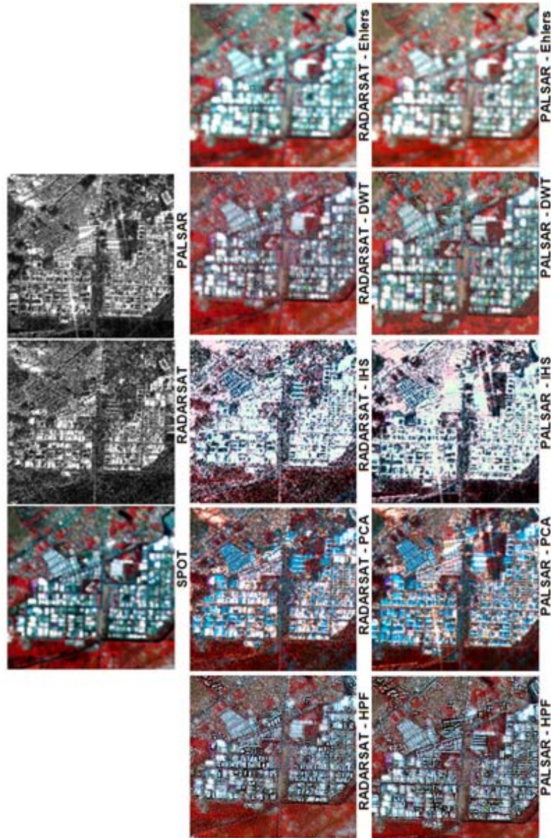
Figure 3 - Comparison of the spectral and spatial effects of the fused SAR-SPOT results for urban areas.
