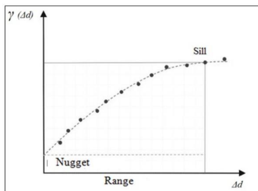
Figure 1: Representation of semivariogram's parameters.
