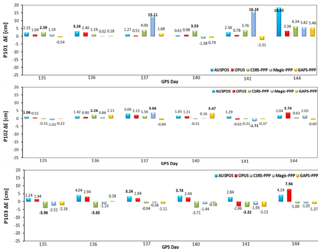
Figure 4: Coordinate differences of East ( \Delta E ) component between the Bernese software and web-based services over 6 days for P101, P102 and P103
