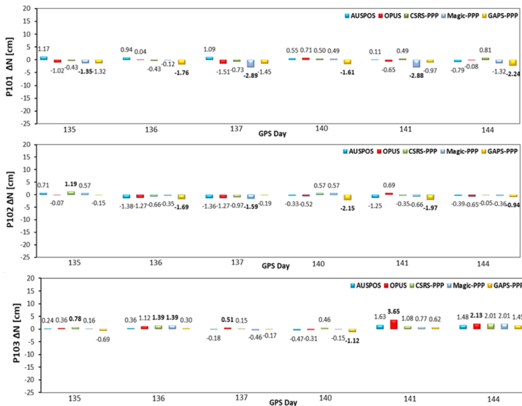
Figure 3: Coordinate differences of North ( \Delta N ) component between the Bernese software v5.0 and web-based services over 6 days for P101, P102 and P103
