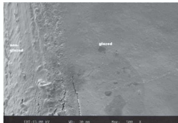
Figure 1. Boundary region between the glazed side and the non-glazed side, before denture insertion. Original magnification X500.
