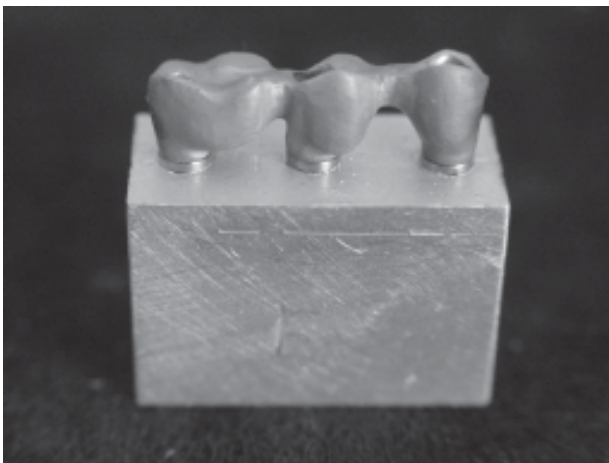
Figure 3. Frameworks placed on metal matrix for SEM analysis.
