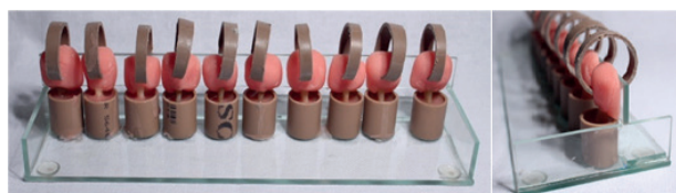
Figure 1. Device for inclusion of tooth roots in PVC tubes and produced perpendicularity between the tooth and tube base.
