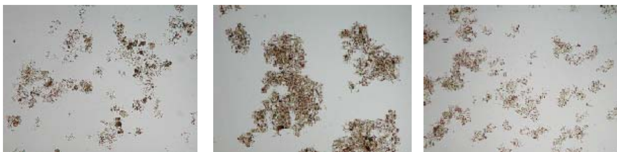
Figure 2: Microscopic images in bright field (total magnification 120x) of microbial flocs from wastewater treatment plants, (a) flocs from REPAR sludge, (b) flocs from Ilha do Governador sludge, (c) flocs from CIBA sludge
