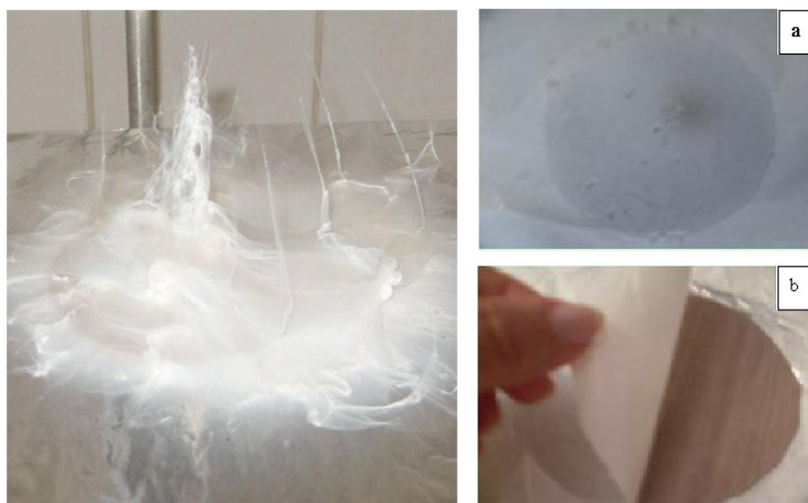
Figure 3: On the left, a picture of the membrane made from the 6D-blend solution (with NaCl); on the right, the membrane made from blend 4B (without salt), a) picture taken immediately after the electrospinning process, b) releasing the membrane from the mold.
