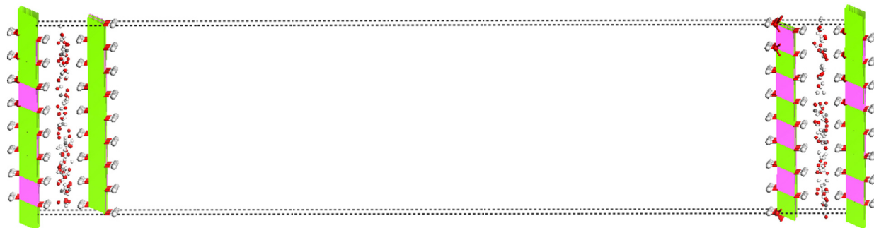
Figure 3: Simulation cell with 72 Å between layers to represent the hydrotalcite pore. White – H; Red – O; Pink – Al; Green – Mg.
