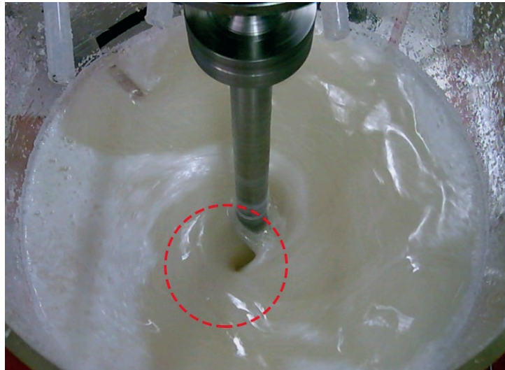
Figure 10. Eccentric vortex observed in experiment (TXL impeller, N = 150 rpm, \mu = 75.3 mPa·s, C_0 = 0.05 L/L).
