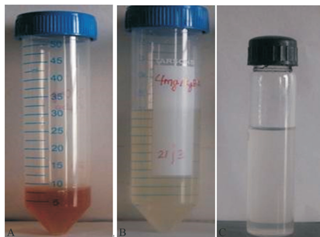
Figure 1 - (a) Colour change in \text{AgNO}_3 solution after addition of 5 mL (0.4%w/v) extract and 5 mL of 1.5 M NaOH (b) Natural biowaste peel extract of P. granatum (0.4% w/v) prepared by 70% ethanol in soxhlet extractor at 40 °C for 48 h (c) 2 mM \text{AgNO}_3 aqueous solution.
