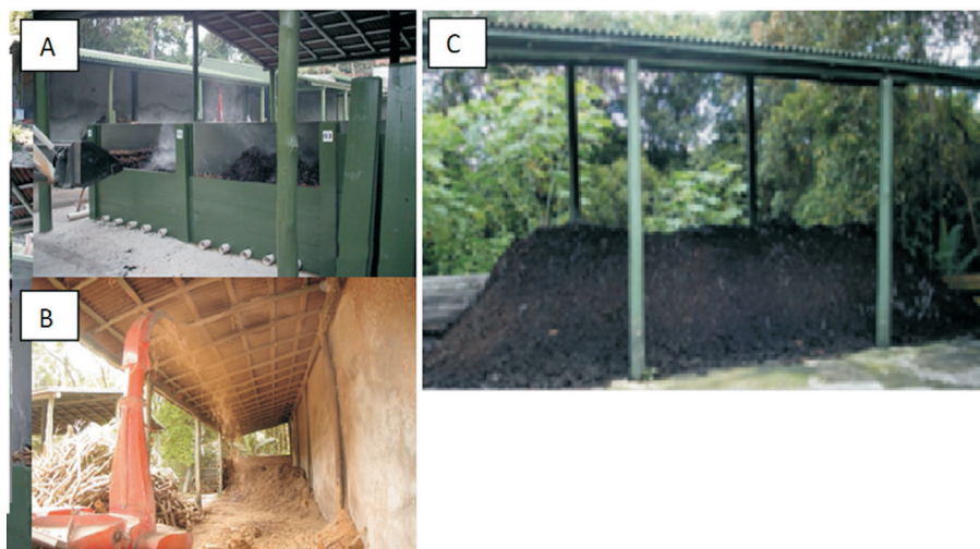
Figure 1 - Partial view of the Organic Composting Production Unit (OCPU) of São Paulo Zoological Park Foundation. (A) Aerobic composting process in the thermophilic phase; (B) grinding of plant matter from the Atlantic Rain Forest; (C) maturation phase of the composting process.
