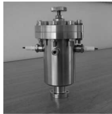
Figure 2. High pressure gas chamber constructed for the TCABR pellet injector: (a) schematic drawing and (b) the chamber in its final form.
