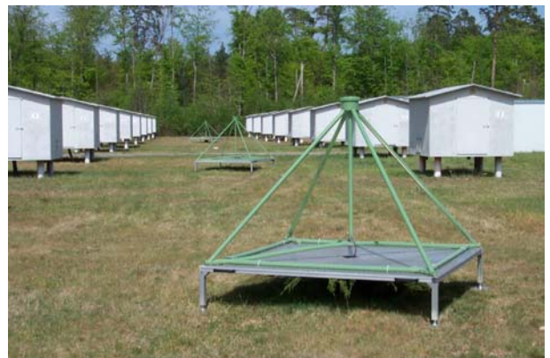
FIG. 1: Inverted V dipole antenna for the LOPES experiment integrated into the KASCADE array. Only two 'legs' of the dipole are equipped with antennas, such that only one polarisation in east-west direction can be measured. In the background one can see some scintillator sampling detectors in wooden housings on the campus of the Forschungszentrum Karlsruhe.
