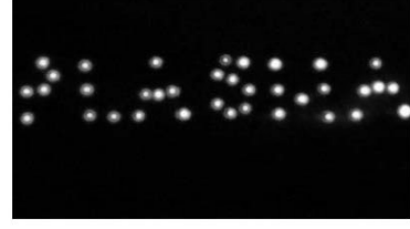
FIG. 4: V - I characteristics for closed MHC dc operated in Ar, with hole diameter of 500 \mu\text{m} at a pressure of 30 and 40 Torr, for 1 and 4 holes. Closed microhollow cathode, Cu anode 100 \mu\text{m} thick, operated in Ar. Hole diameter D = 500 \mu\text{m} . Mica spacer 250 \mu\text{m} thick and cathode cavity deep of 200 \mu\text{m} . In the right a digital photography shows an association of MHCs ( D = 200 \mu\text{m} ).
