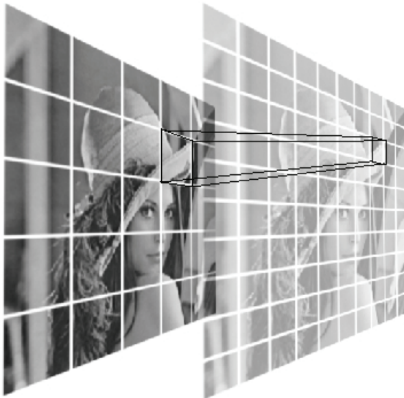
Figure 1 – In Partitioned Iterated Function System, self-similarity is sought between larger portions of the image (Domain blocks) and smaller portions (Range blocks clusters).
