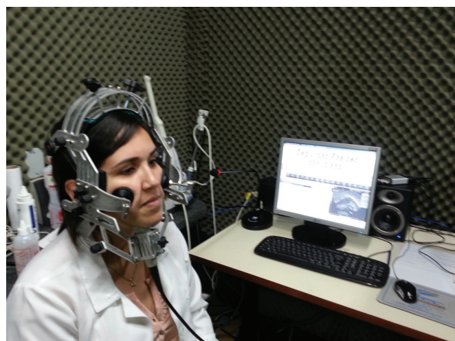
Figure 1. Collection of data: individual sitting down using the head stabilizer with the ultrasound transducer attached to the submandibular region
