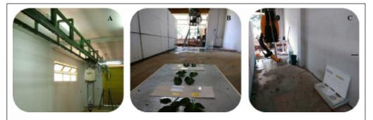
Figure 1 - Rail structure used to move the sprayers (A) and positioning of the sample units used for hydraulic (B) and pneumatic sprayers (C). Source: (A) Quirino, 2010. (B) and (C) the authors.
