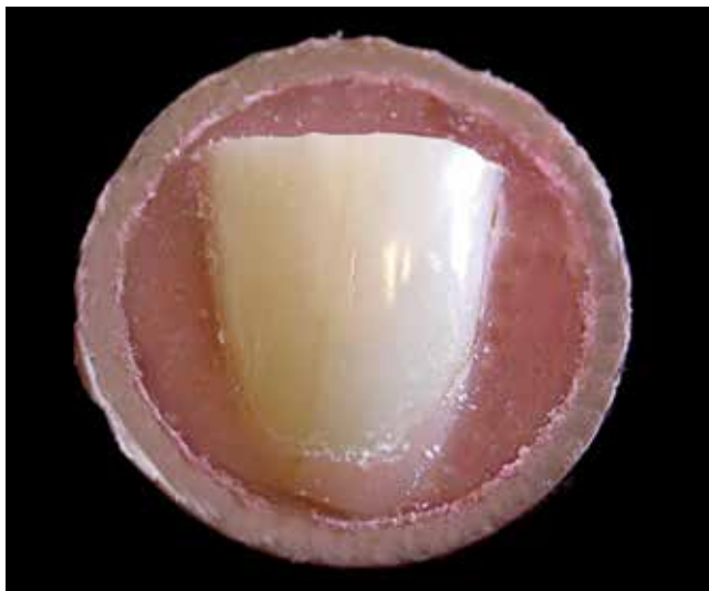
Figure 2 - Bovine tooth sectioned at the cervical third of the root and at the incisal third of the crown and included in acrylic resin.
