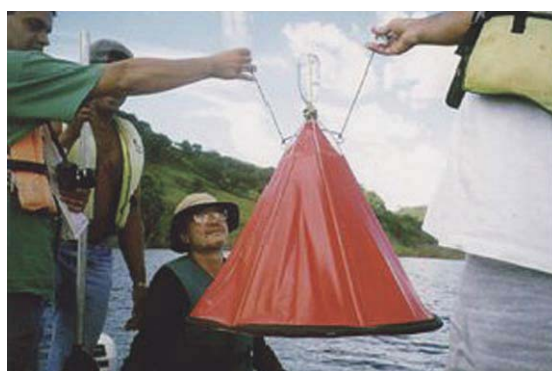
Figure 9 – Greenhouse gases emissions measurement in hydroelectric plants made by Coppe-UFRJ and by USP- São Carlos.
