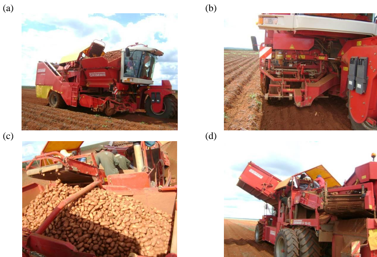
FIGURE 1. Self-propelled potato harvester Grimme SF 150-60. (a) Harvester overview. (b) Intake. (c) Deposit. (d) Moving floor bunker.
