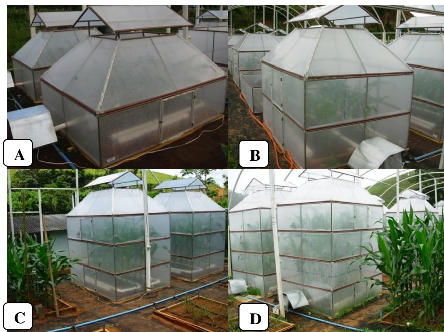
FIGURE 2. Open-top chambers with the addition of modules to follow the crop growth: A - 1 module, B - 2 modules, C - 3 modules, and D - 4 modules.
