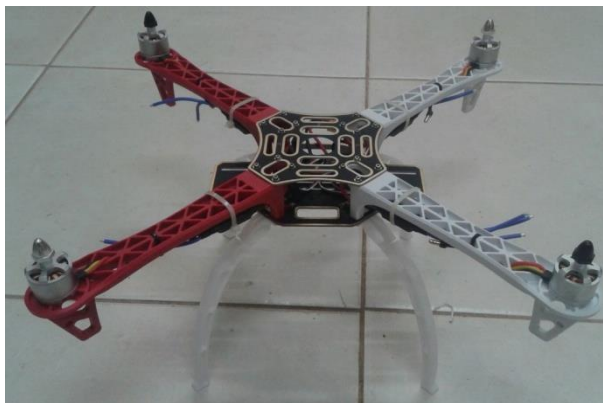
FIGURE 3. RPA assembly structure, ready to receive the sensors.
