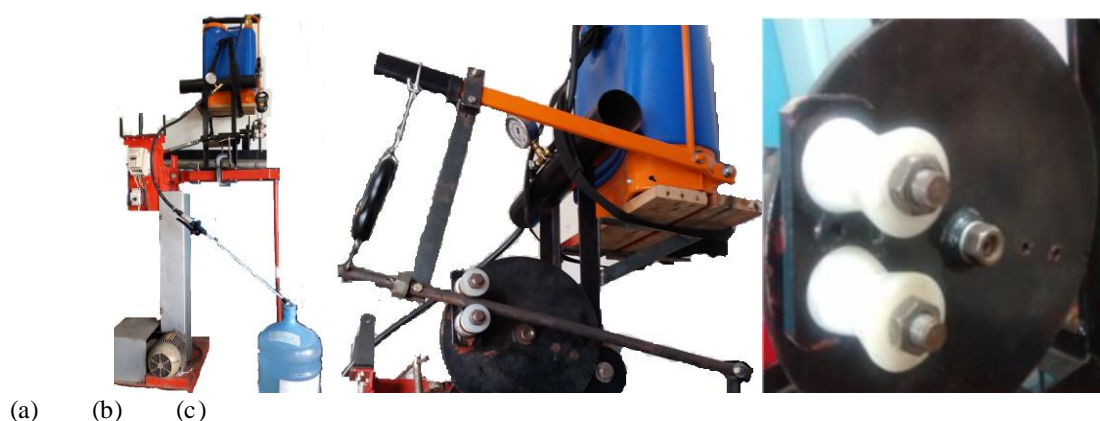
FIGURE 2. Test Rig (a), crank rod system type Scotch Yoke Mechanism ® (b) and “V” mobile roller mechanism (c).
