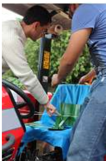
FIGURE 2. Device for determining the SIP positioned on the seat of a sampled operating station.
