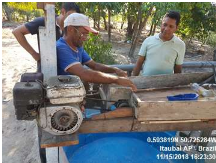
FIGURE 2. Equipment used by the farmer to grate cassava.
