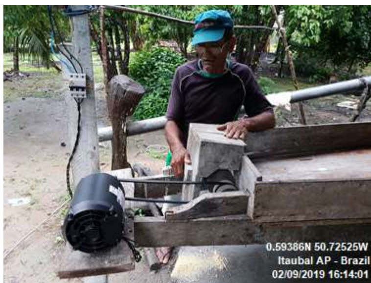
FIGURE 3. Cassava grater equipped with an electric motor instead of the gasoline engine.
