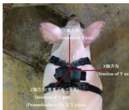
FIGURE 2. Direction of the back-mounted triaxial accelerometer. The X-axis pointed from the left to right side of the pig's body, the Y-axis pointed from the tail to head of the pig, and the Z-axis was perpendicular to the XY plane.
