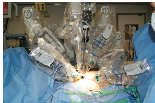
Figure 2. External aspect of the operative field: DaVinci™ robotic system docked to the patient
