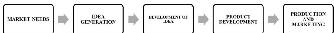
Figure 2. Linear Reverse Model ( Market Pull or Demand Pull ). Source: Adapted from Rothwell (1994) and Barbieri (2003).
