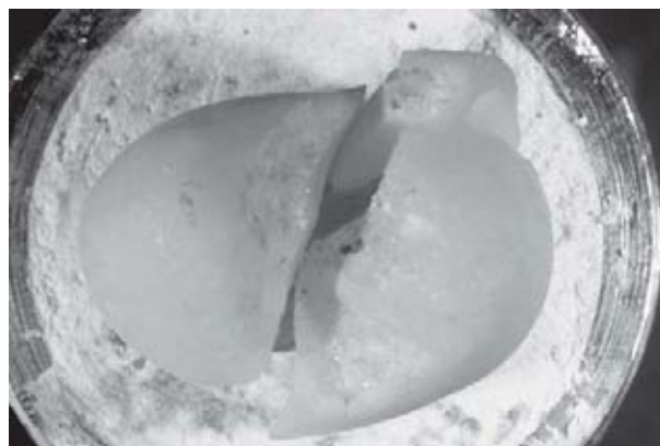
Figure 3- Fractured specimen after application of compressive load
