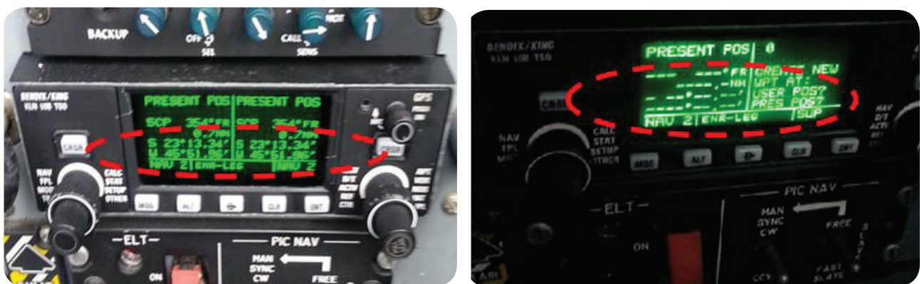
Figure 9. Aeronautical GPS receiver under spoofing.
