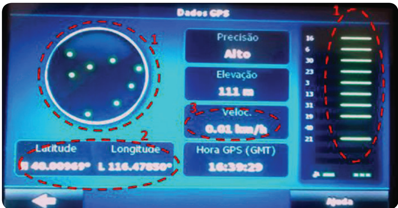
Figure 6. Automotive receiver under static spoofing.
