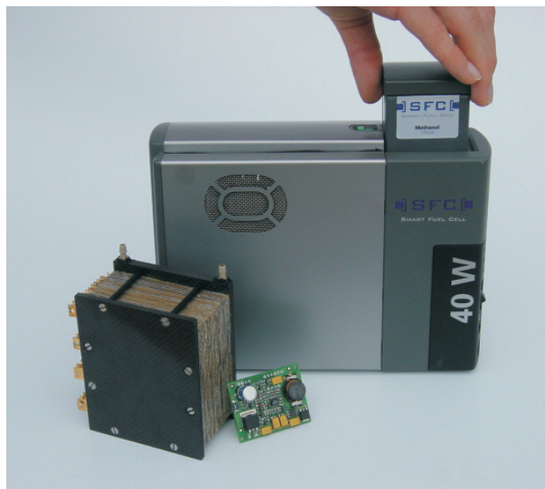
Figure 13. The 40 watt PEM DMFC fuel cell system from Smartfuelcells, Brunnthal/Germany, working at ambient air, 200 mA/cm 2 at 400 mV cell voltage, 12 volt stabilized, 60 °C, 1 mg/cm 2 PtRu(50:50), 1 Wh/cm 3 methanol. 19
