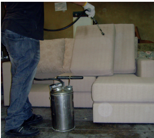
Figure 1 – Manually-compressed resin spraying system with a discharge valve. Note the presence of droplets on the lens of the camera as a result of the product spray.
