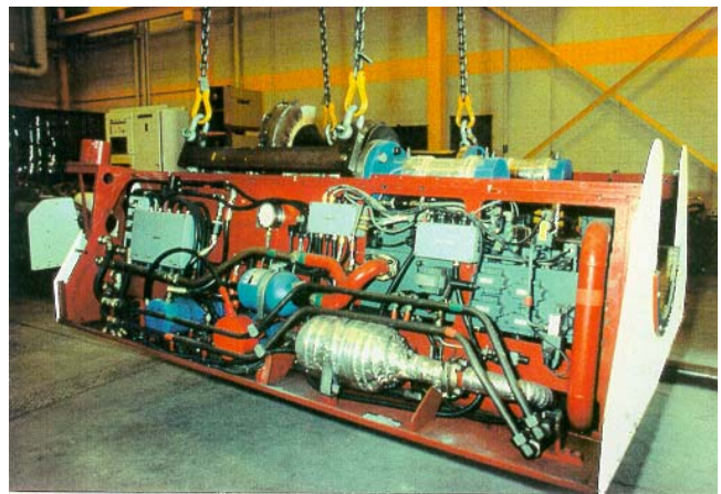
Figure 15. MIAB NPS 12 welding head.
