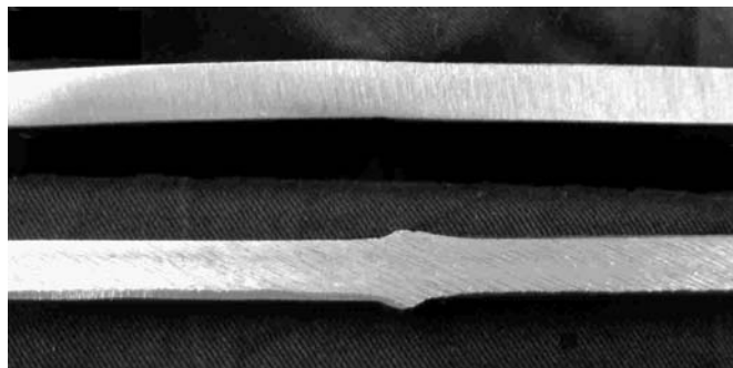
Figure 13. Control of weld flash in spinduction welding.
