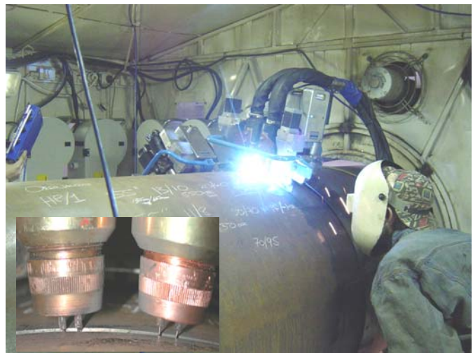
Figure 4. Arrangement of CAPS welding torches and system mounted on RMS welding systems mechanised welding bug.
