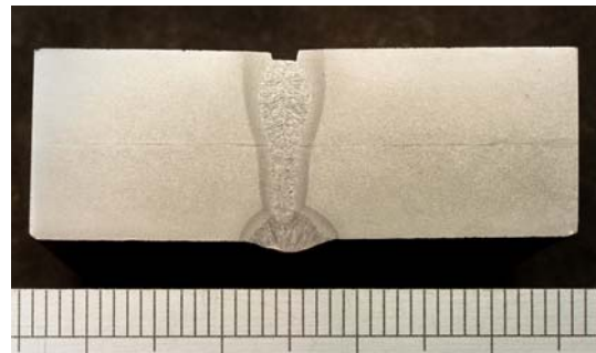
Figure 9. IWM root pass with HL-GMAW first fill.
