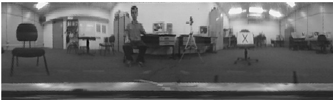
Figure 15. Panoramic image created by a direct mapping of the pixels of the image acquired by the hyperbolic mirror.
