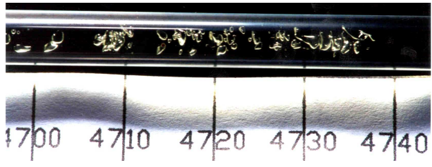
Figure 13. Flow pattern at z about 4.7 m for test 18.
