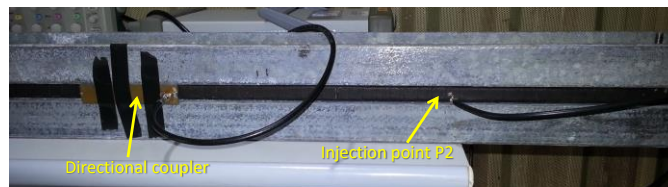
Fig. 21. Injection point P2 and directional coupler over the bar in experimental setup.
